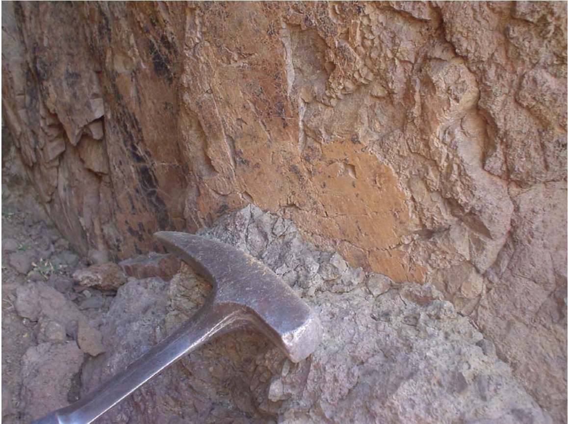
Figure 5.18. Exposures of discrete, planar fault surfaces are rare in the DMQ. This photograph is the only example found of such a feature. The magnitude of offset on this structure is unknown but it cuts through a lithic-rich Challis Volcanic Group rock. The structure strikes to the south dipping 60^\circ to the west. Slickenlines trend toward the northwest plunging steeply. This may suggest the last movement of the fault was obliquely to the northwest.
